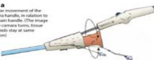
D_2 With the knob on handle B, tool B (the gripper) can be opened and closed, when pushed back, the heating is activated. This way branched veins can be separated.
