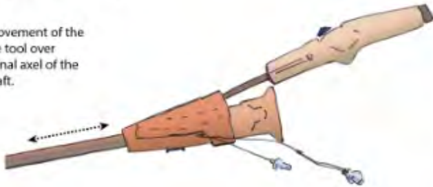
A_4 Translation of position of the complete tool (without pivoting).
